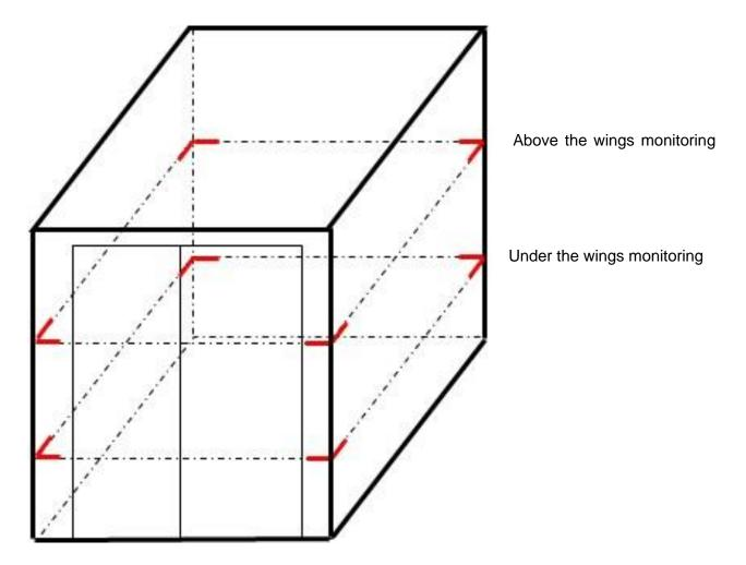
Airplane hangars are a versatile and demanding application. Because of its dimensions, the maintenance activities taking place and objects which may cause obscuration of the flame detector and friendly fires. Correct positioning of the detectors is from utmost importance, to monitor every potential fire risk. The Sense-WARE IR3 and UV/IR flame detectors are suitable for this application, with a combination of a good sensitivity, a fast response and good false alarm immunity.
