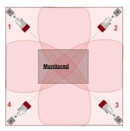
Be aware of the shadow effect. You can avoid the shadow effect by putting another detector in the opposite corner. This second detector also works as redundant device in case the other detector is blocked.
